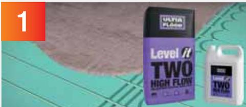
Apply Ultra Floor Level-it 2 two part smoothing compound over entire floor area, making sure all voids and gaps are completely filled, the levelling compound should encapsulate the whole floor and cover the board with a 5mm layer on top (if tiling). **If fitting Vinyl this must be a minimum depth of 10mm.**
