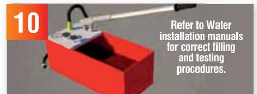
10 Upon completion of the underfloor heating pipe circuits - ensure all pipe work is pressured tested (conforming to BS EN 1264). The mixing valve temperature should not be set above 55 degrees Celsius for floating floor or solid floor systems.
