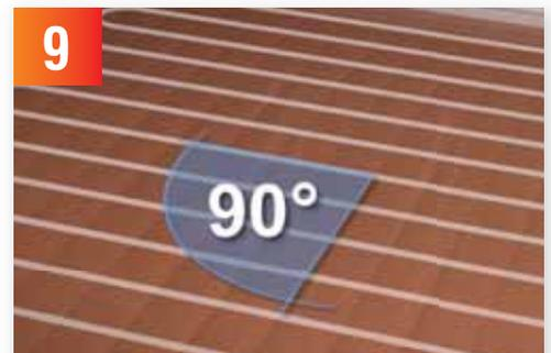
9 Ensure that when installing floorboards they are positioned at a 90° angle to the pipe direction.
